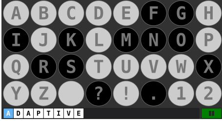
Figure 2: Virtual keyboard. During the stimulation the target is highlighted in blue below the keyboard.
