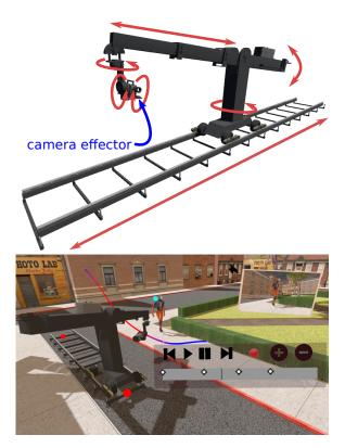
Figure 11: Our system allows the interactive and key-framed manipulation of complex camera rigs (here a Technodolly rig) defined through a list of constrained degrees of freedom (in red in the top image). The camera effector (in blue) is directly controlled by the user.
