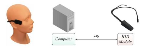
**Fig. 1.** HID module placed in the head (*left*). Simplified architecture of the Human-Computer Interface device in USB connection mode (*right*).
