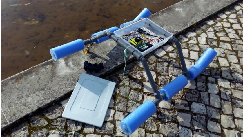
Fig. 4. Working prototype for a low-cost unmanned surface vehicle, developed by the research team from IPT.
