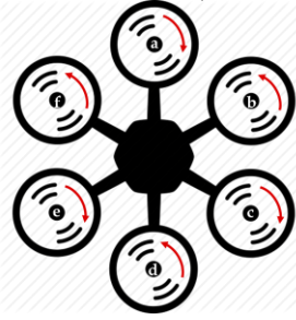
Fig. 3. A simple hexacopter with rotors labeled from a to f (PNPNPN configuration).
