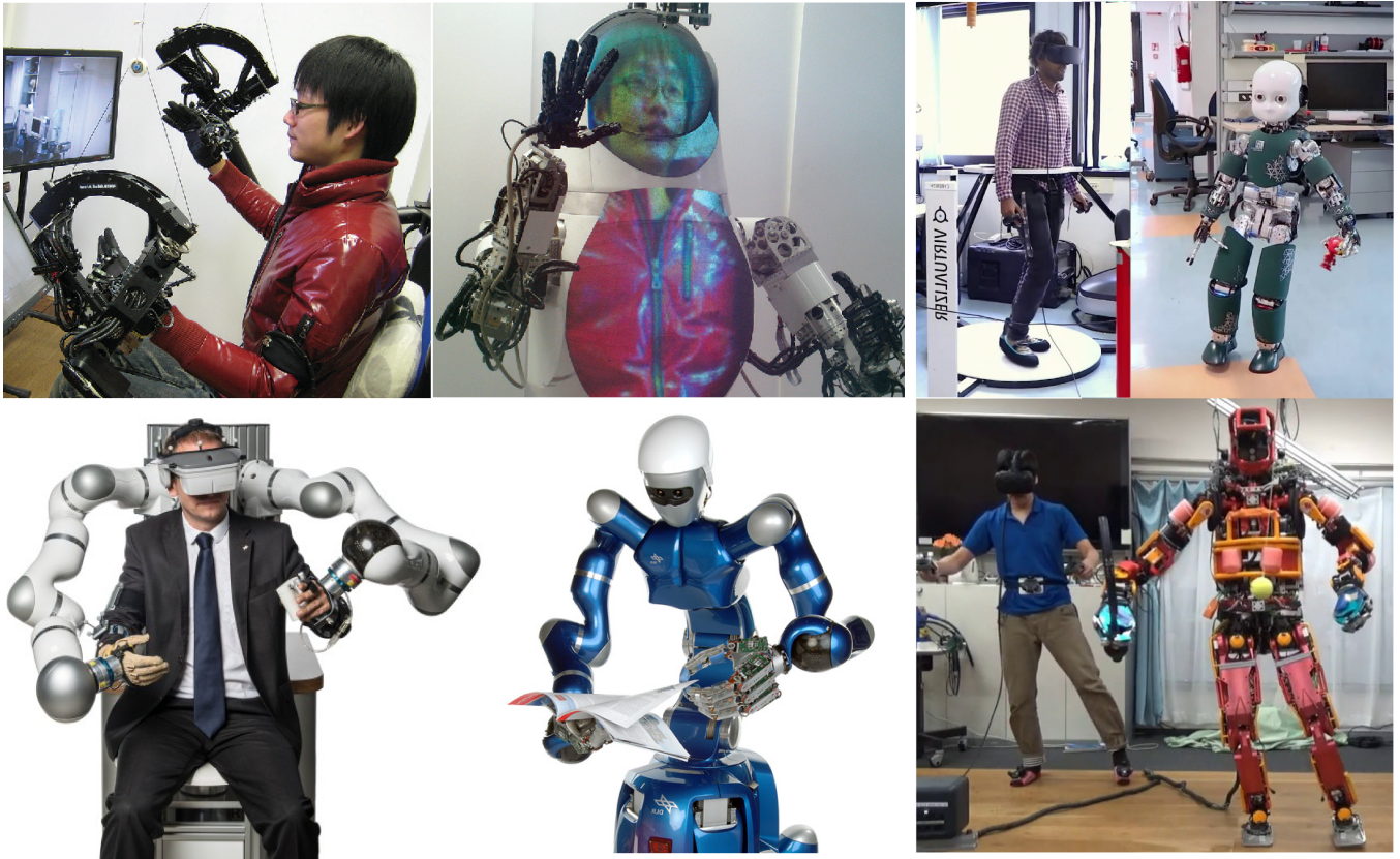
Fig. 3: State-of-the-art in humanoid teleoperation. Top-left: TELESAR II [9], a mutual telexistence system; Bottom-left: Immersive teleoperation of the Justin robot with haptic feedback at the hands [10]; Top-right: Telexistence of the iCub robot with a VR walking platform [13]; Bottom-right: Dynamical whole-body teleoperation of the JAXON robot [14].
