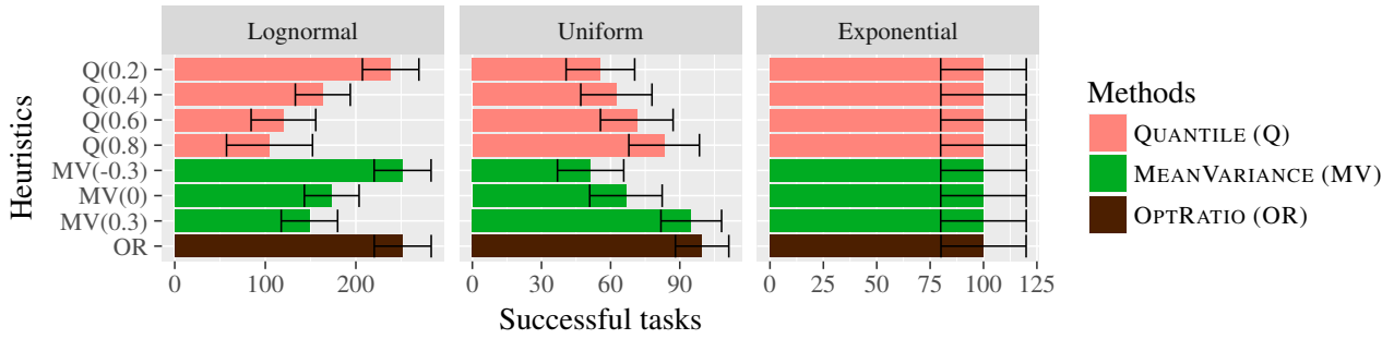
Figure 2. Number of successfully executed tasks for each heuristic with three distributions (lognormal, uniform, exponential) of same expected value \mu = 1 , with a budget and deadline b = d = 100 (which means that a single machine is enrolled). Each heuristic is run 100,000 times for each scenario. The error bars are computed with the mean plus/minus two standard deviations of the number of successes. The lognormal distribution has parameters \alpha \approx -1.15 and \beta \approx 1.52 to have an expected value \mu = 1 and a standard deviation \sigma = 3 , and the optimal cutting threshold for OPTRATIO is l \approx 0.1 ). The exponential distribution has shape \lambda = 1 and the cutting threshold is arbitrarily set to l = 2 . The uniform distribution has parameters a = 0 and b = 2 , and the cutting threshold is l = 2 .
