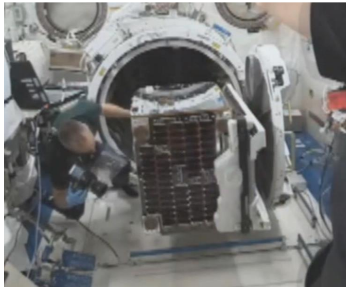
Figure 6: RmoveDEBRIS installed on the airlock sliding table
