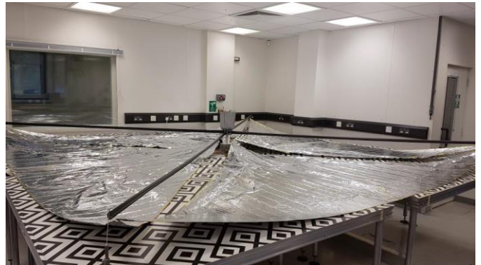
Figure 31: Deployment test of the DragSail for the SSO-A mission
