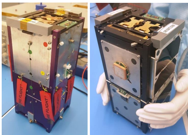
Figure 14: CRS insertion on to CubeSats. This figure shows DS-1 (left) and DS-2 (right) with the CubeSat Release Systems (CRS) attached (on top).
