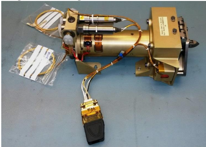
Figure 19: FM Harpoon Payload . Showing the harpoon payload (no MLI) without the harpoon target or casing.
