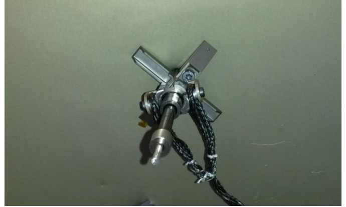
Figure 24: Harpoon Impact. This figure shows a harpoon impacted into a target.
