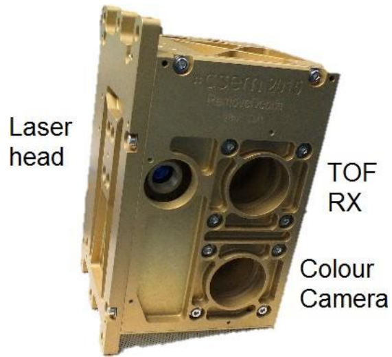
Figure 28: VBN: Sensor PFM.
