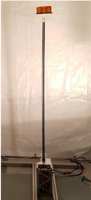
Figure 23: FM Boom - Deployed. This figure shows the harpoon target assembly (HTA) and the boom fully deployed to 1.5 m with gravity assistance.
