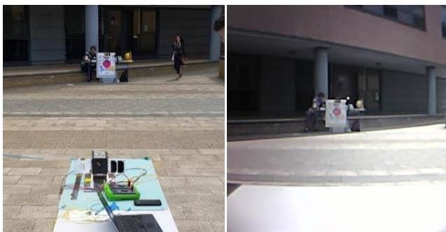
Figure 9: FM DS-2 and ISL SEET. Full end-to-end DS-2 CubeSat (containing camera, sensors and inter-satellite link) test transmitting data back to a simulated platform. Left: test setup with CubeSat shown on surface. Right: view from CubeSat camera (as transmitted back to the platform).
