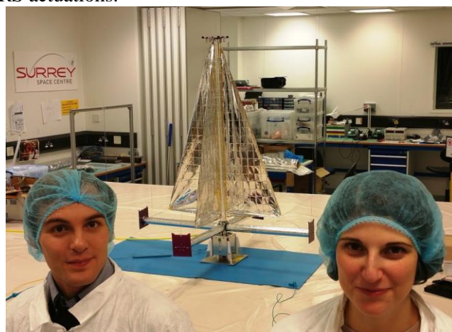
Figure 11: DS-1: FM CubeSat SEET Inflation. This figure shows the DS-1 CubeSat under a final deployment test as part of the SEET.
