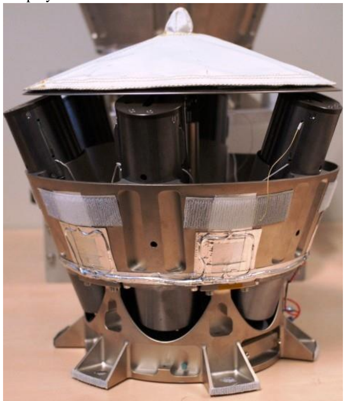
Figure 17: FM Net. This figure shows the final net flight model with ejection springs unloaded.
