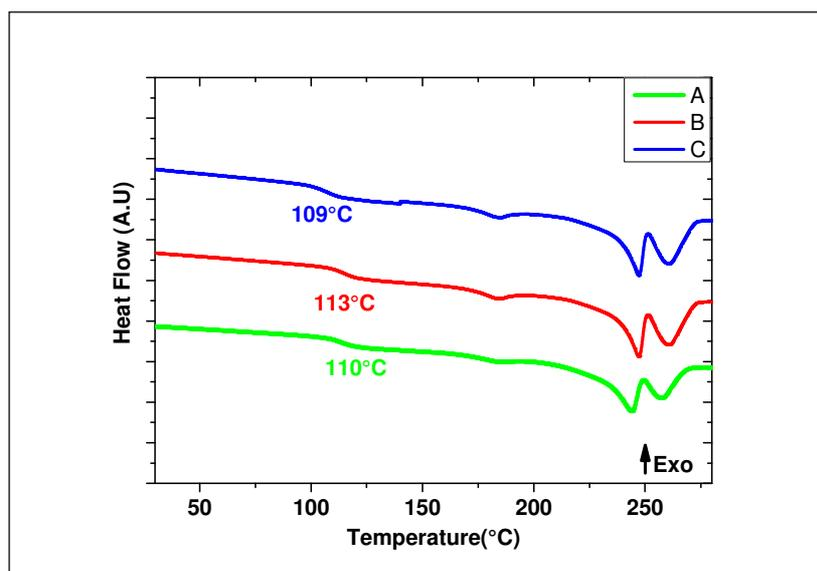
**Figure 18:** DSC scans (2st heating) of continuous glass fiber reinforced parts (PPA/CA bi-component systems injected at 280 °C +60% by weight of glass fibers). Sampling at (A) the beginning of the flow, (B) in the middle area and (C) at the end of the flow.
