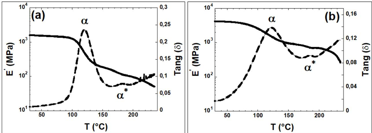
**Figure 20.** Evolution of storage modulus and  $\tan(\delta)$  as a function of temperature for (a) a neat PPA matrix, and (b) glass fiber-reinforced PPA composites obtained at a reaction temperature of 280 °C.
