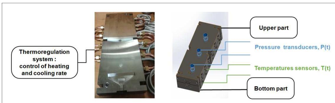
Figure 4. Design (left) and realization (right) of the instrumented and thermoregulated RTM mold.
