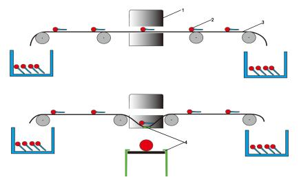
1. X-ray detector, 2.Lollipop, 3.Conveyor belt, 4.Guide roller added
