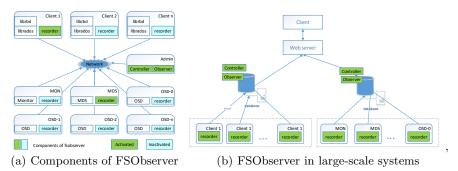
Fig. 1. Architecture of FSObserver
