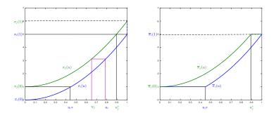
Figure 2.1: Capillary pressure curves (left) and truncated capillary pressures curves (right)
