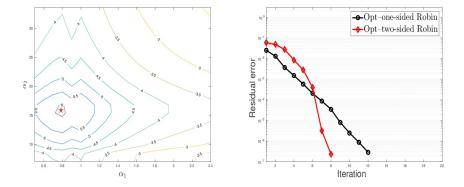
Figure 6.9: Example 2: Left: Level curves for the residual error obtained after 8 iterations for various values of the parameters  $\alpha_1$  and  $\alpha_2$ . The red star shows the optimized parameters. Right: The convergence curves of the optimized Schwarz method with one-sided optimized Robin conditions and two-sided optimized Robin conditions.
