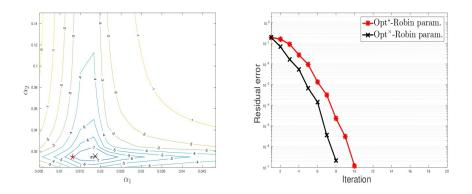
Figure 6.5: Example 1: Left: Level curves for the residual error obtained after 10 iterations for various values of the parameters  $\alpha_1$  and  $\alpha_2$ . The star (in red) marked the parameters obtained with the minimization process of the convergence factor applied to the linearized problem which is close to the best one marked by times symbol (in black). Right: The convergence curves.
