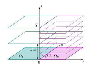
Figure 5.2: Nonconforming time grids between two subdomains  $\Omega_1$  and  $\Omega_2$
