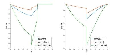
Figure 6.4: Example 1. Error in saturation along a line orthogonal to the interface, nonconforming and conforming (coarse and fine) time-steps. Left  $T = T_f/20$ , right,  $T = T_f$ .
