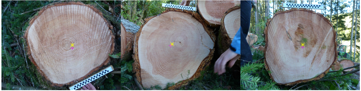
Figure 4 — Some cases where our method fails to detect precisely (less than 5mm) the pith. In red cross results of the first step, and in yellow star the results after the second step. The first two cases show the same log end but with a slight rotation. The error can be explained by a high presence of sawing marks, knot near the pith and green dirt near the pith. The third failure can also be explained by a high presence of sawing marks.
