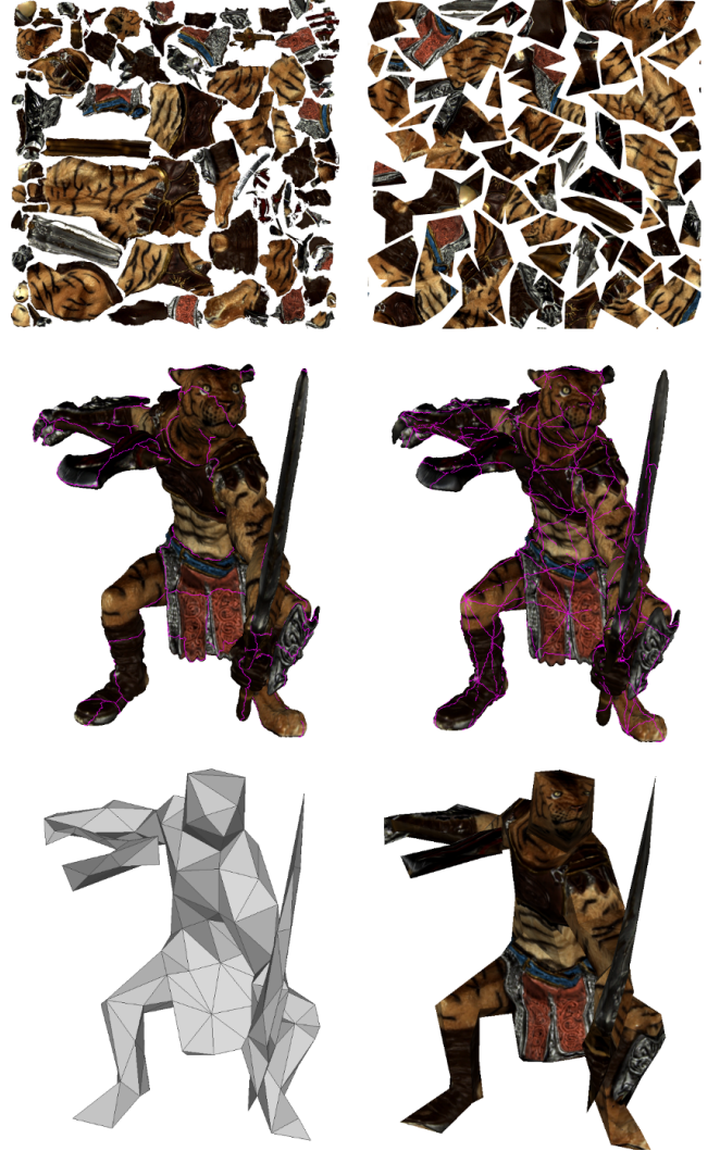
Figure 5: Re-atlasing. Top: input atlas and new atlas. Middle: input seams and seams after re-atlasing via the abstraction mesh. Bottom: abstraction and textured abstraction mesh.
