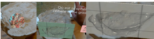
Figure 8: Left : Random dot-mask rendered on the 3D printed urn. Middle: cut plane moved with hand position. Right : Point on cut plane moved with head orientation.
