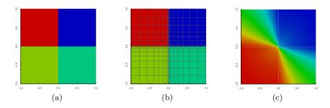
**Fig. 5.** Kellogg's test problem: (a) The computational domain and the four subdomains, (b) the graded meshes of the four subdomains, (c) the contours of  $u_h$  solution.
