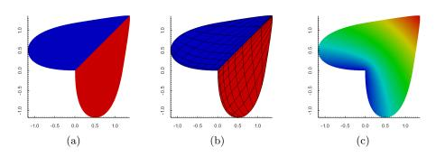
**Fig. 4.** Heart shape problem: (a) the computational domain and the subdomains, (b) the graded meshes of the two subdomains, (c) the contours of  $u_h$  solution.
