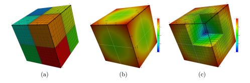
Fig. 7. Cube with interior singularity: (a) the decomposition of  $\Omega$  into 8 subdomains with the graded meshes of the subdomain, (b) the contours of the solution  $u_h$ , (c) the variance of the  $u_h$  contours around the singular point.
