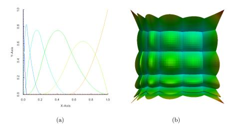
**Fig. 3.** Basis functions on the graded mesh  $T_{h_{i_{\zeta}},\widehat{\Omega}}^{(i_{\zeta})}$ : (a) The 1d bases on  $\mu=0.6$  grading, (b) The 2D bases on  $\mu=0.6$  grading.
