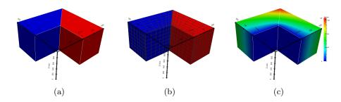
**Fig. 8.** 3d L-shape test: (a) The domain  $\Omega$  with the corners and the edge boundary singularities, (b) The graded meshes of the two subdomain, (c) The contours of  $u_h$ .
