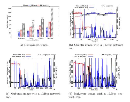
Figure 2: Deployment times and resource usage using standard Docker.
