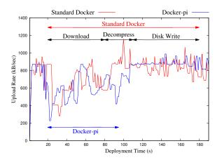
Figure 11: Upload throughput of the Apache web server.
