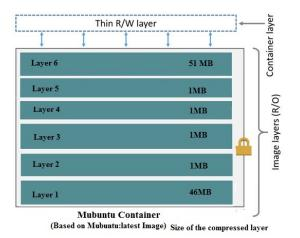
Figure 1: Structure of the "Mubuntu" container image.
