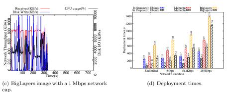
Figure 9: Resource usage and deployment time with Docker-pi.
