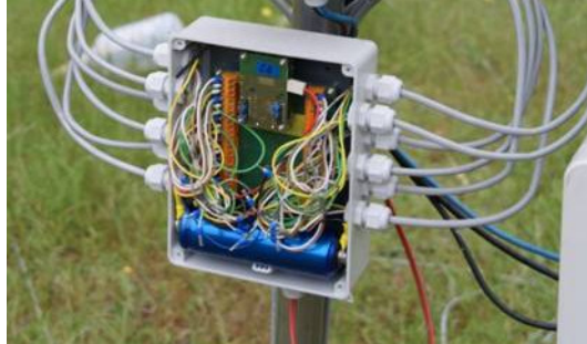
Fig. 6. Since the embedded analog-to-digital converter suffered from precision problems, and could not connect several sensors, we developed our own ADC board and connected up to 12 sensor to it (showed in this photo). However, we had to still manually calibrate the new ADC and did not know if the calibration is needed after some time, e.g. when the temperature changes. Therefore, in the next project we used sensors based on the digital SDI-12 protocol.
