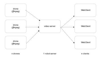
Fig. 2. Multimedia transmission architecture.
