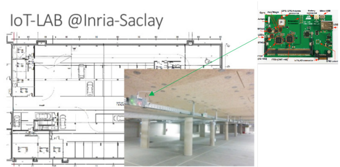
Fig. 6. Measurements are done on a network of 37 “A8” nodes on the Saclay IoT-Lab testbed, deployed in a parking structure.
