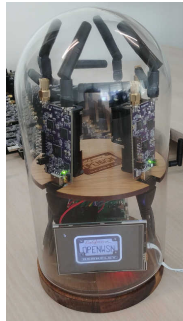
Fig. 3. At OtBox: a Raspberry Pi, 4 OpenMote B boards, a screen and a QR code in a glass dome.
