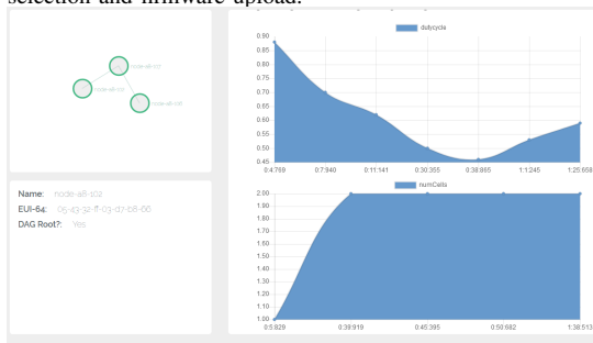
Fig. 4. Screenshot of the real-time KPI monitoring as the experiment progresses. The figure on the bottom depicts the increase in assigned bandwidth once the node has joined the network. The figure on the top shows how duty cycle varies depending on the phase.
