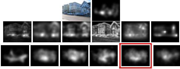
Fig. 4: Predicted saliency maps for the different tested saliency models. From left to right, first row: original image and ground truth; second row presents the predictions from RARE2012, Hou, AWS, SUN, GBVS, SAM-VGG. From left to right, third row presents the predictions from SalGAN, RI-M1, RI-M2, RI-M3, FT-M1, FT-M2. The red frame indicates the prediction having the highest CC.
