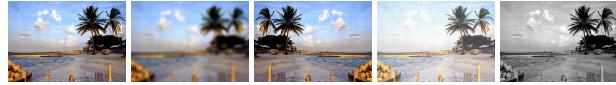
Fig. 3: Different data augmentation methods. From left to right: original, blurred, flipped, noisy and grayscale image.
