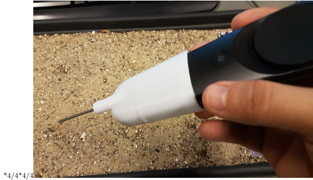
Fig. 7. The needle used for the experiment, made from a 3D printed mount and a nail and attached with a bolt in the loop designed for the wrist strap.
