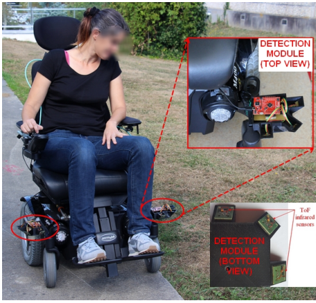
Fig. 10: On-going test on a real power wheelchair.
