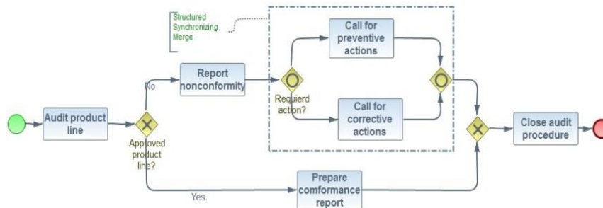
Fig. 3. Structured synchronizing merge in BPMN
