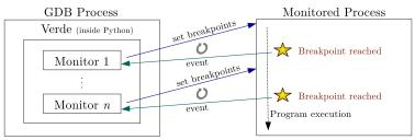
Fig. 23. Instrumentation in Verde
