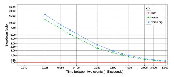
Fig. 27. Instrumentation overhead with Verde. raw (red) is the execution of the program without Verde. verde (green) is the execution with Verde. The overhead includes the breakpoint-based instrumentation. verde-arg (blue) is the execution with Verde, and one parameter is used in the produced events. The overhead includes the instrumentation and the time used to retrieve one value per event.
