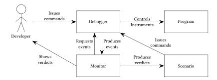
Fig. 1. Overview of Interactive Runtime Verification. The developer issues commands to the debugger, the debugger controls and instruments the program, the monitor requests program events to the debugger and issues verdicts to the scenario and the scenario applies developer-defined reactions.
