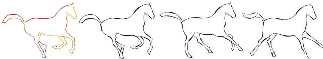
Figure 9.7: 2D curve tracking by active contours (Bénard et al., 2012) — The contour curves extracted from a galloping horse are tracked by active contours (left) ensuring a coherent parameterization of the strokes (right) during the animation.
