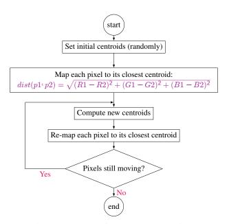
Fig. 2: Flowchart of the K-means algorithm
