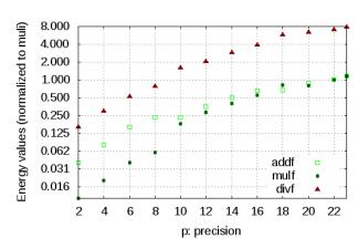
Fig. 3: Normalized energy values for different precisions
