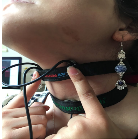
Figure 1. Position of the emitting diodes and photosensitive sensor. The subject presses each of the two diodes against her neck.
