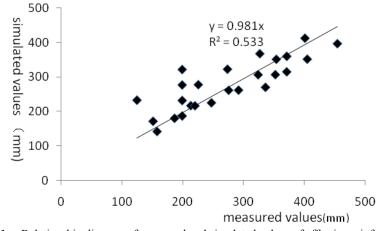
**Fig.1.** Relationship diagram of measured and simulated values of effective rainfall As can be seen from the figure 1, the square of the correlation between simulated and measured value of effective rainfall is 0.533. Thus the correlation coefficient is 0.73. It shows that the measured and simulated of effective rainfall has a good correlation. Based on the above results, it can be drawn that the water balance calculation method of effective rainfall is valid.
