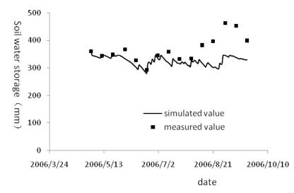
Fig.2. Comparison Chart of measured and simulated values of soil water storage without irrigation
