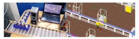
Fig. 5. Physical testbed with cosmetic products, RFID tags and readers and virtual testbed implemented by QUEST
