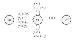
Figure 5: Computing a greatest common divisor
