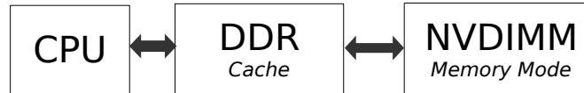
Figure 2: 2-Level-Memory mode (2LM) uses DDR as a Memory-side Cache in front of the Memory Mode part of NVDIMMs exposed as normal volatile memory.
