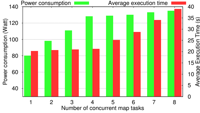
Fig. 1. Observations for both (i) the average task execution time and (ii) power consumption when varying the number of concurrent running tasks: Map task when running WordCount application (compute-intensive tasks). Using the model developed in Section 4.1, we obtain: \mathcal{P}_{\text{static}} = 65W and \mathcal{P}_{\text{dyn}} = 17W .
