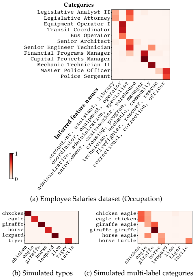
Fig. 4: Gamma-Poisson factorization gives positive and sparse representations that are easily interpretable. Examples of encoding vectors ( d=8 ) for a real dataset (a) and for simulated data (b and c) obtained with a Gamma-Poisson factorization. The x -axis shows the activations for each dimension with their respective inferred feature names. Figure 13 in the Appendix shows that other encoders fail to give such an easily-understandable picture.
