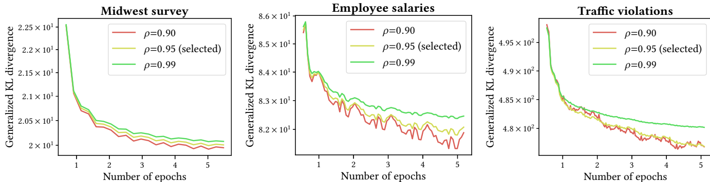
Fig. 9: Convergence for different discount factor values for the Gamma-Poisson model. In all experiments, the value \rho = 0.95 is used, as it gives a good trade-off between convergence and stability of the solution across the number of epochs.
