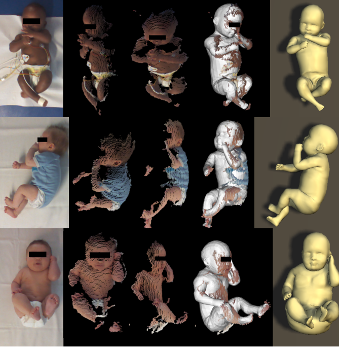
Fig. 4. SMIL registration results. From left to right: RGB, point cloud, point cloud (other view), point cloud with registered SMIL, rendered registration.
