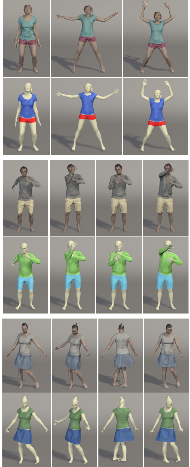
Fig. 10. Results of the multi-cloth alignments with shape underneath presented in pairs of (scan, result). From top to bottom we present different garments: t-shirt with shorts, jersey with shorts and t-shirt with skirt.
