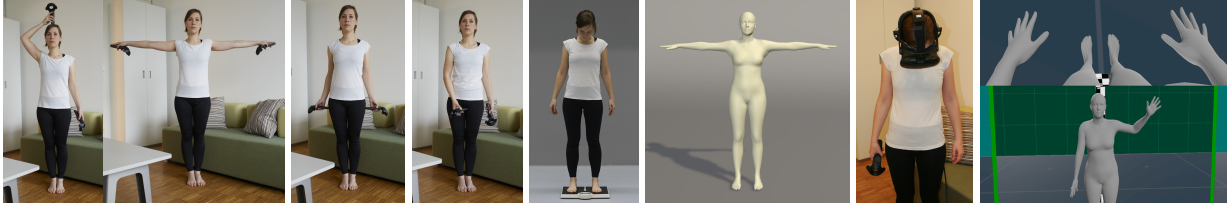
Fig. 1. The Virtual Caliper. A novice user takes 3D measurements of her body using the wand controllers of the HTC Vive in just under 5 minutes by following simple instructional videos. Additionally, the user is asked to enter her weight and gender. The Virtual Caliper immediately produces a rigged 3D model with exactly the dimensions of the measured person. The rigged 3D model can be used straight away in Unity or exported for use in other 3D modeling packages. We illustrate a virtual mirror application where the user can look down and experience her body in VR.
