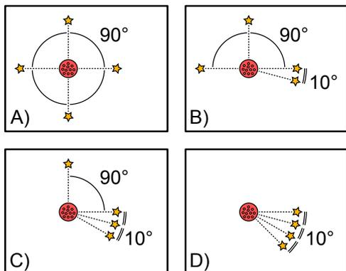
**Fig. 1:** The four sound source configurations considered in our simulations. Note: stars represent sound source locations. All the sources and the spherical microphone array are at the same height. Across all the examples, the position of sources with similar type was the same.
