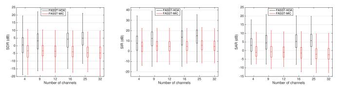
Fig. 2: Comparing FASST performance in regards of number the used microphones/channels.
