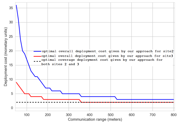
Figure 1.8: Optimal deployment cost given by our model depending on the communication range of nodes.
