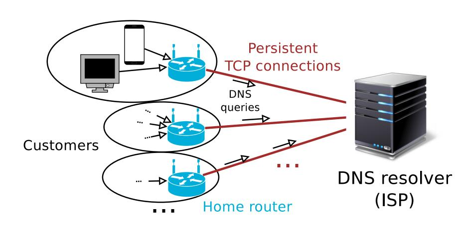
We setup a large-scale testbed on Grid'5000 [1] to implement this deployment model. Each physical machine hosts several Virtual Machines (VM) acting as clients. A dedicated machine hosts the DNS resolver.
