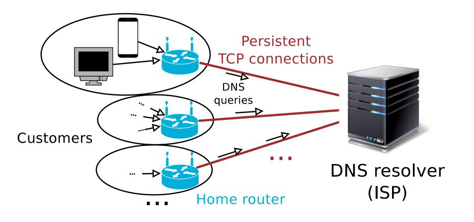
We setup a large-scale testbed on Grid'5000 [1] to implement this deployment model. Each physical machine hosts several Virtual Machines (VM) acting as clients. A dedicated machine hosts the DNS resolver.
