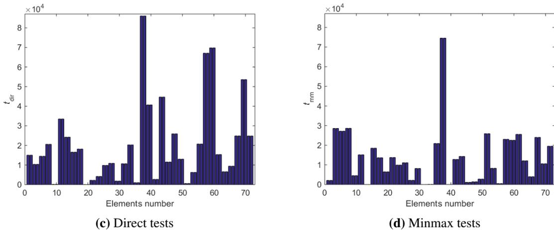
**Figure 8:** Test case 2: Localization for damaged cables 37 and 38, using 15 modes.
