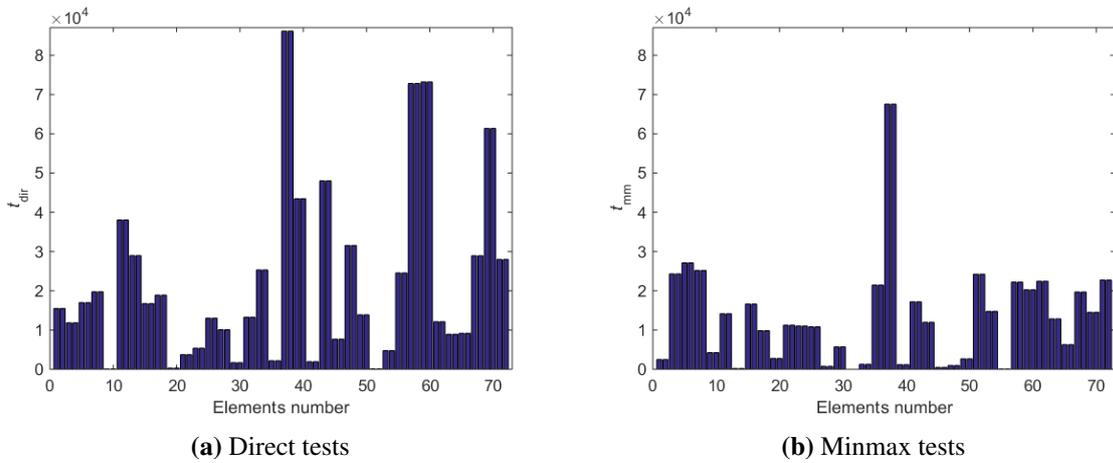
**Figure 7:** Test case 1: Localization for damaged cable 37, using 15 modes.
