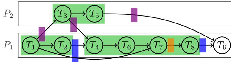
**Figure 5.** Blue *induced* checkpoints are used to isolate task sequences on a processor (labeled in green, such as the sequence  $T_4, T_6, T_7$  and  $T_8$  on  $P_1$ ). Finally, additional checkpoints can be added inside an idle-free task sequence through a dynamic programming algorithm: the orange checkpoint corresponds to such an addition.
