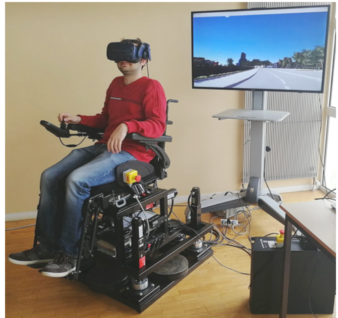
Fig. 1: The Power Wheelchair Simulator (PWS): motion platform and 3D scene displayed through HMD for an immersive experience in Rennes city
