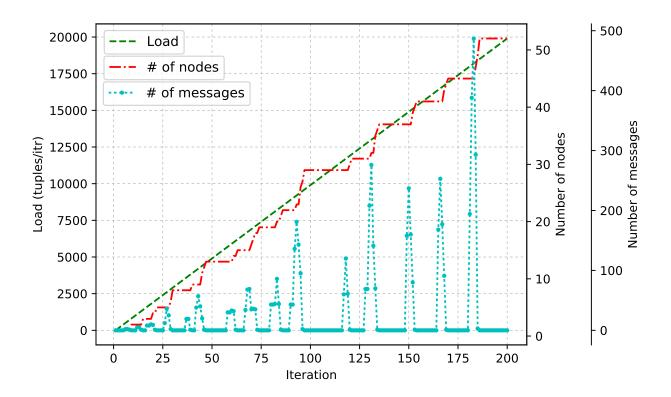
Figure 6: Traffic when facing a monotonically increasing load.
