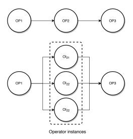
Figure 1: Scaling out a simple application.
